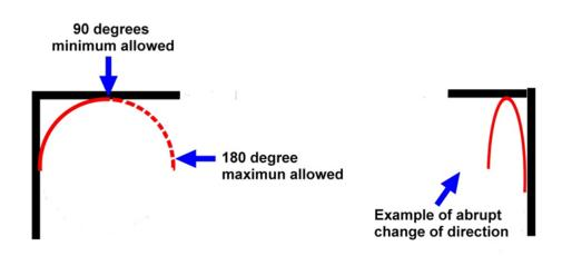
Although the 180 degree ear is allowed the 90 degree is preferred.
